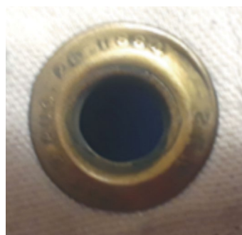
Figure 15. A brass U.S. Navy grommet stamped with date and size. Photo by author.
